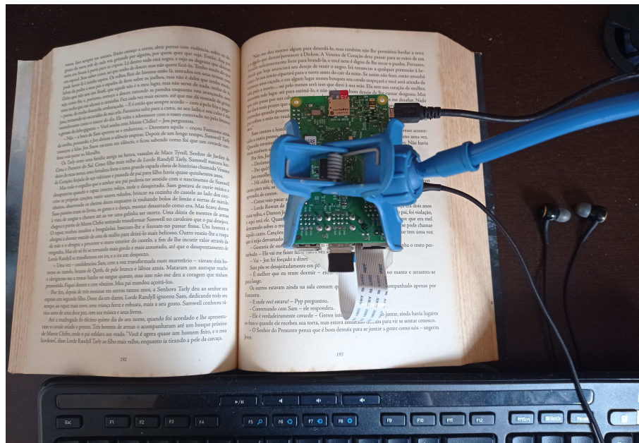
Figure 12 – Book2Speech supported by a cell phone holder above the book to be scanned. The system waits for the capture or cancel command to perform an action.
