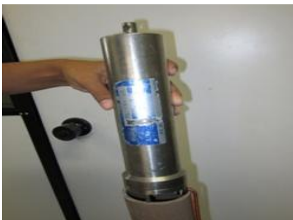
Figura 14- Sensor OBS (modelo Turbinfinity- ATU75W)
